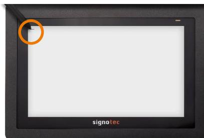
After rebooting, the LED lights up orange. Two intersecting lines (like a plus sign) will appear on a white background in the upper left corner of the display.
