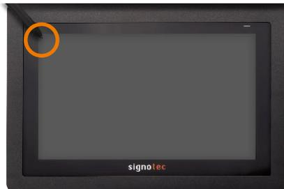
Disconnect the pad from the power supply. Touch the **upper left corner** of the display with the pen. While holding the pen, reconnect the pad to the power supply.
